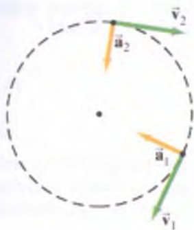
6-rasm. Aylana bo'ylab tekis harakat uchun \vec{a} va \vec{v} lar doimo perpendikulyar
