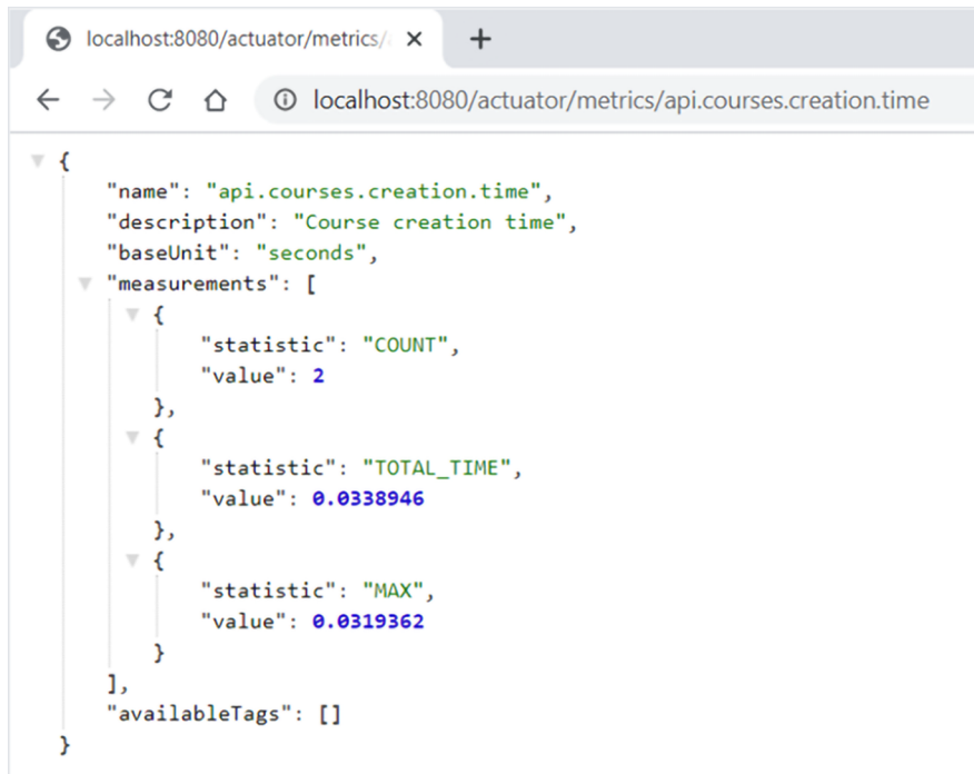
Figure 4.22 Outcome of the api.courses.creation.time custom metric. The baseUnit indicates the unit for the metric and provides an option to customize the unit for the metric.
