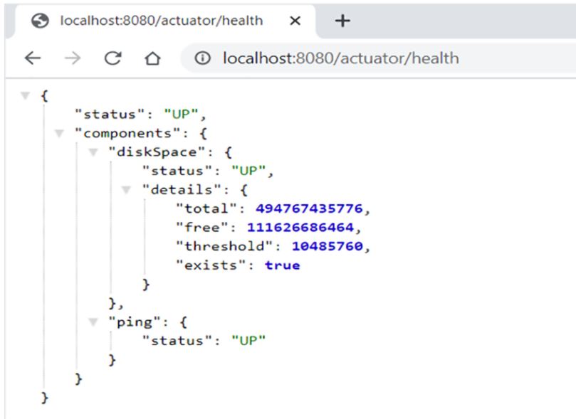
Figure 4.6 Spring Boot Actuator health endpoint with show-details always configuration
