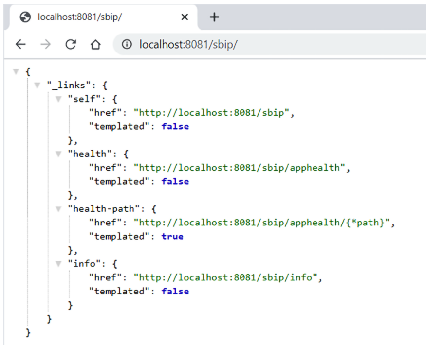
Figure 4.5 Spring Boot Actuator endpoint discovery page with custom content. In this example, the /actuator context is customized to /sbip . The management server port is 8081, whereas the application port is 8080.
