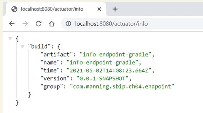
Figure 4.12 Accessing build information in a Spring Boot Gradle application through info endpoint
