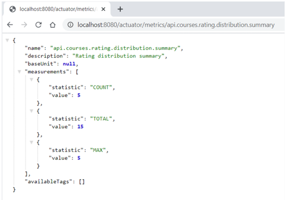
Figure 4.23 Outcome of the api.courses.rating.distribution.summary custom metric. The COUNT property indicates how many courses have been created. The TOTAL provides information regarding the aggregated value of the rating. Lastly, the MAX property shows the maximum value of a course rating. For demonstration, we've used the course rating in this example. We can also use other details, such as time in units of second and length to capture distribution summary.
