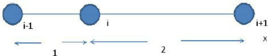
Figure 5.17: Nodal arrangement used to solve problem 5.7.
