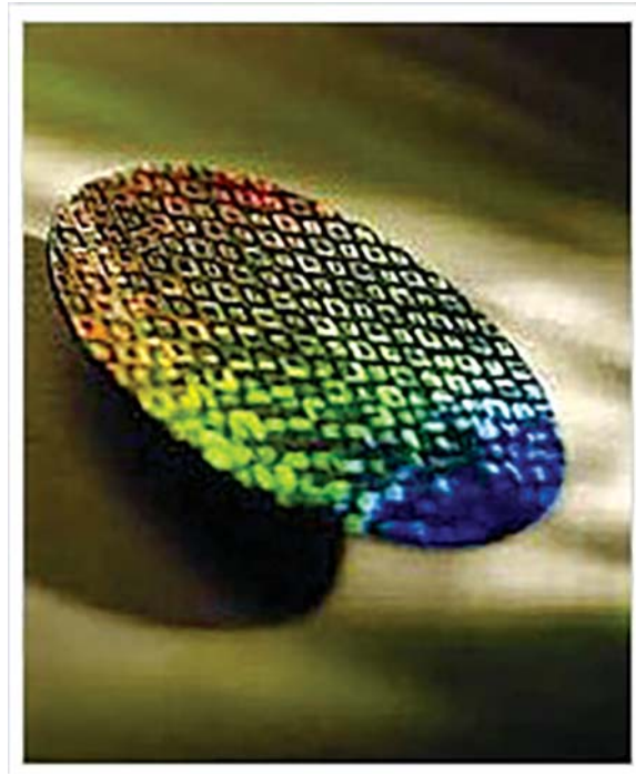
Figure 8.10.1 An etched silicon wafer.
