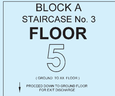
9A EXAMPLE OF A STAIRWAY MARKING SIGN [FLOOR INDICATION BOARD]
