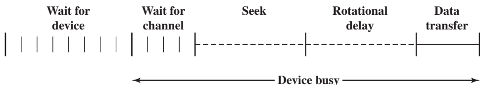
Figure 6.5 Timing of a Disk I/O Transfer
