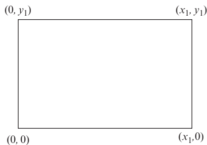
Figure 9.16. A standard rectangle on which four bilinear basis functions can be defined.
